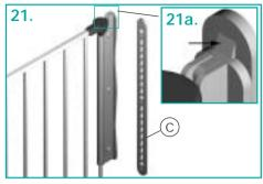
Remove wall plate (C) from assembly by pressing locking tab (21a.) and lifting it off.
